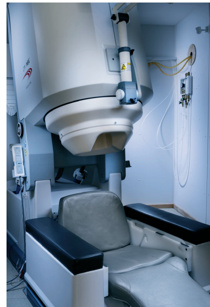
MEG system installed at the Tübingen MEG Center. The MEG system consists of 275 SQUID magnetometers (superconducting quantum unit interference devices) that allow for measuring the magnetic fields generated by the electrical brain activity.
