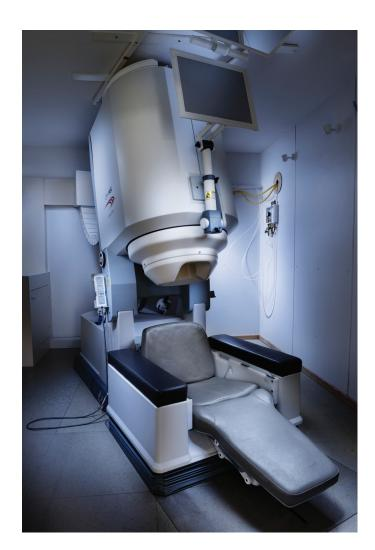
MEG system installed at the Tübingen MEG Center that allows for measuring the magnetic fields generated by brain activity
