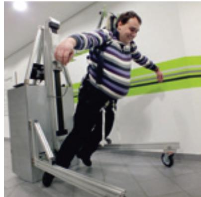
The displayed system allows the application of external mechanical perturbations to the body in order to study the motor control during complex walking.
