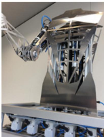
Biorobotic model of the human arm with two joints actuated by five mono- and biarticular pneumatic muscles of different lengths and thicknesses. The robot considers non-linear lever arms and actuators with a nonlinear force-length and force-velocity relation. Built in collaboration with Syn Schmitt, Biomechanics and Biorobotics, University of Stuttgart.
